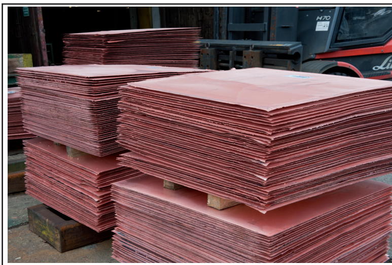
Figure 7.0.1: Copper Cathodes (Source: B.Langner@Aurubis AG, www.aurubis.com )
