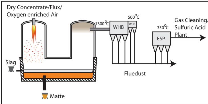
Figure 5.3.5: Principle of the Outokumpu (Outotec) Flash Furnace
